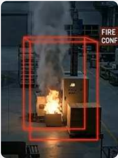
Fire Detection Flame flagged before heat sensors react.
