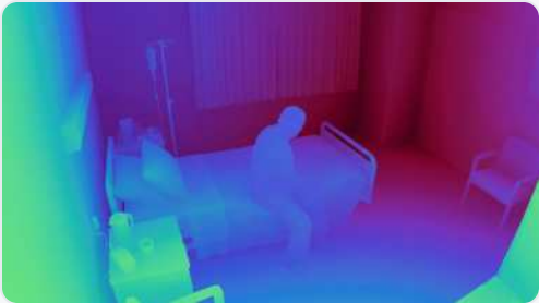
ToF depth sensing: depth data carries no identity
