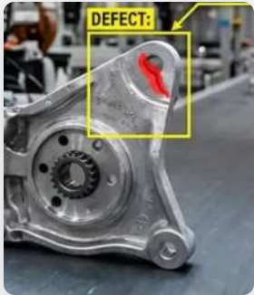
Defect Detection Flaws boxed as parts pass the line.
