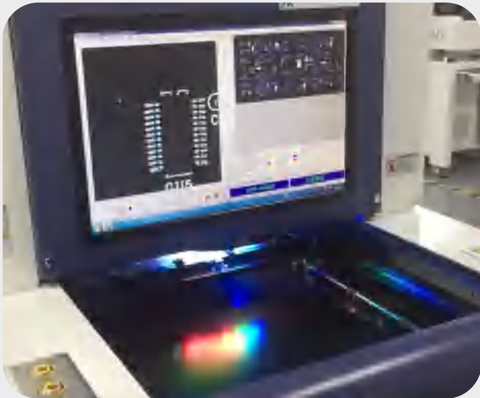
Automated Optical Inspection (AOI)
