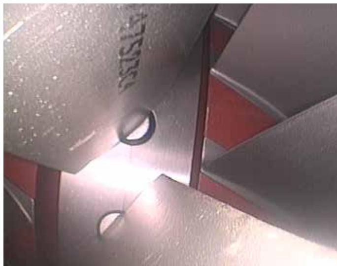
Post 2017: Engine protected with N-hance filters. Borescope has completed after 8,285 operational hours with zero offline water washes.
