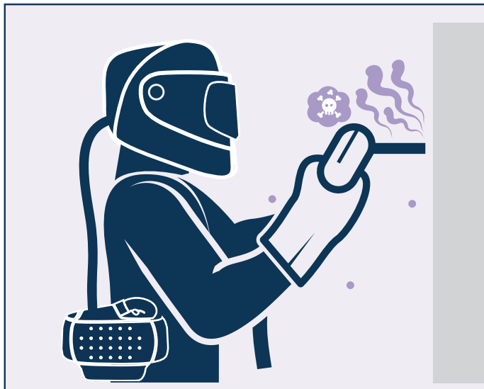
Without On-Gun Fume Extraction
